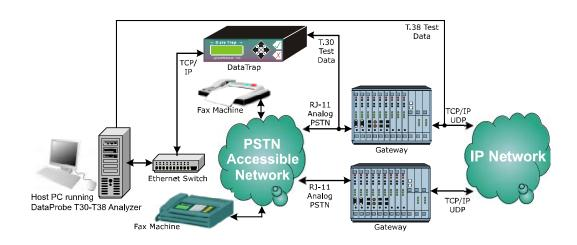
multiple Data Traps and Channel Traps to create an end-to-end test system that plays both the originating and answering terminals in fax sessions that are sent across such complex networks. The system monitors each call, providing T.30 analysis at all modulations, including V.34 and T.38 providing analysis including SIP/H.323. This system identifies protocol violations, fax message degradation and timing errors that result from network signal transport.
